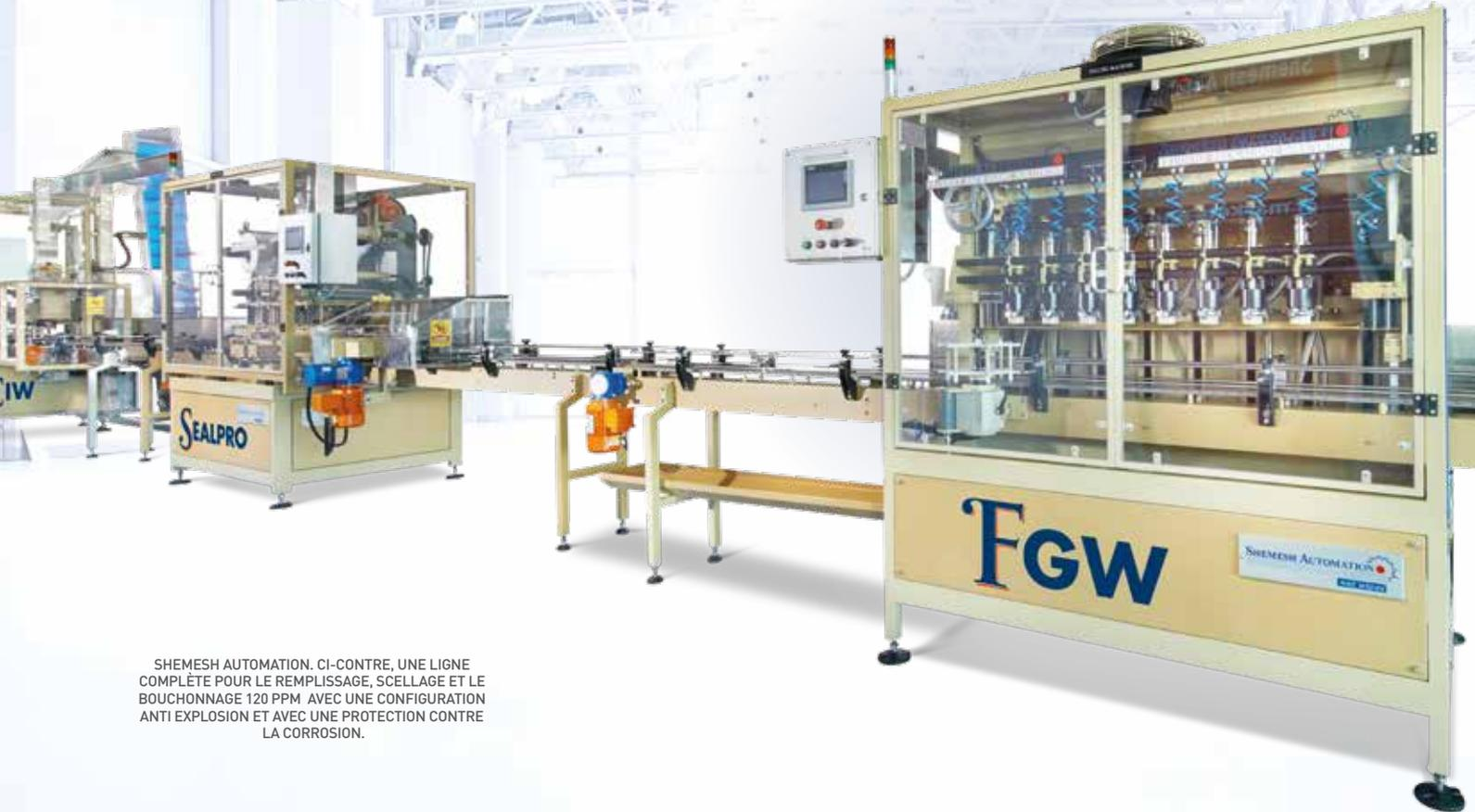
SHEMESH AUTOMATION. CI-CONTRE, UNE LIGNE COMPLÈTE POUR LE REMPLISSAGE, SCELLAGE ET LE BOUCHONNAGE 120 PPM AVEC UNE CONFIGURATION ANTI EXPLOSION ET AVEC UNE PROTECTION CONTRE LA CORROSION.
